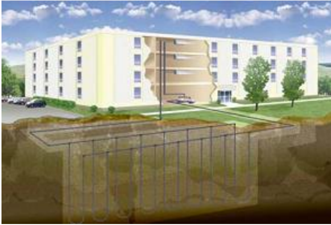
Figure 10 –Conceptual Vertical Loop System
